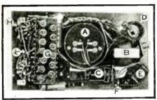
Behind-the-panel view showing the arrangement of parts and wiring. At A, meter; B, power transformer; C, 6C5 tube used as rectifier; D, potentiometer for controlling balancing voltage; E, filter choke; F, ohmmeter and capacity meter adjusting rheostat; G, resistor subpanel, carrying the wire-wound resistance voltmeter; K, rotary switch, (volts, ma., capacity, etc.).
